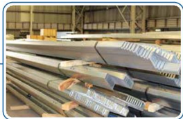
Galvanized Purlins & Zinc Alum Panels
